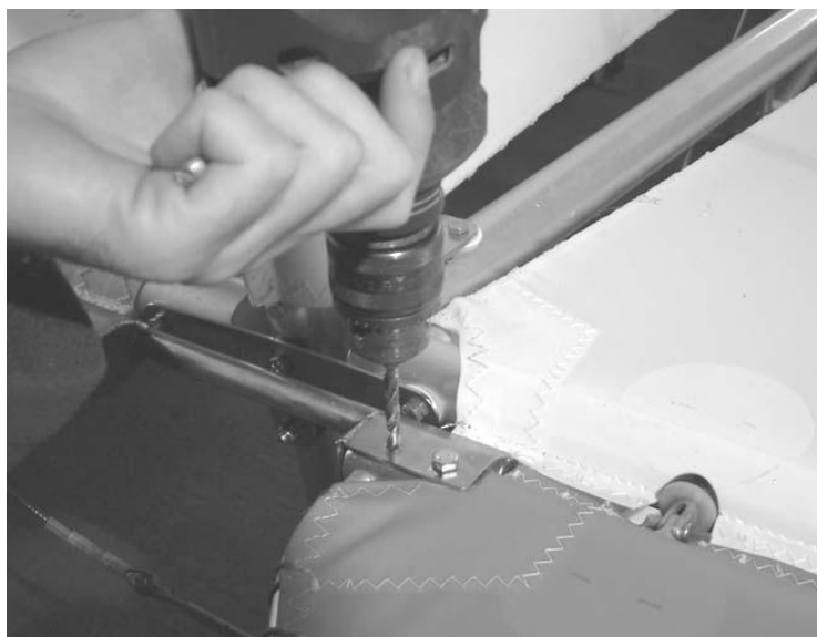
Figure 109 drilling the elevator halves.
