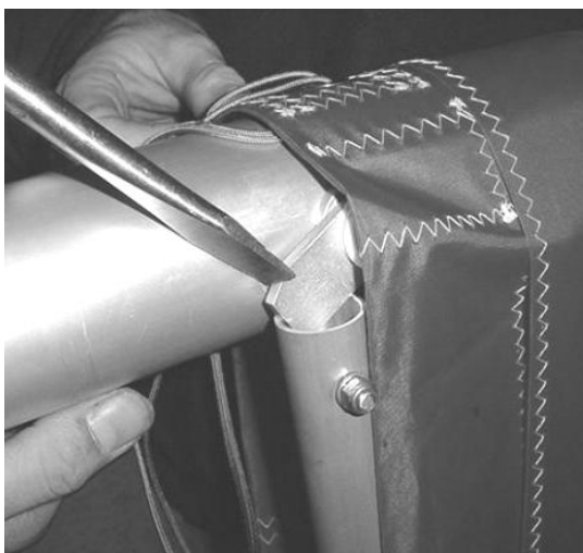
Figure 185 fitting the compression tube.
