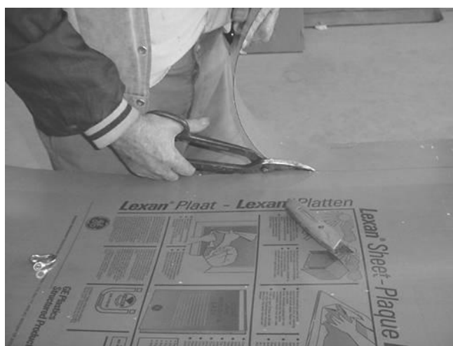
Figure 301 cutting the Lexan to the pattern.
