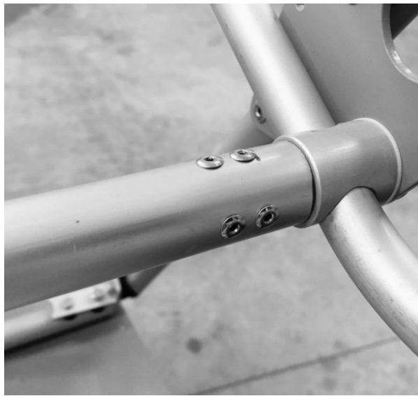
Figure 201 throttle torque-tube rivets.
