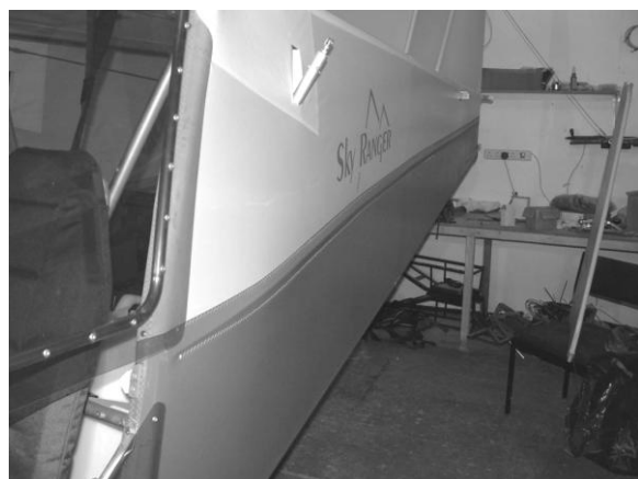
Figure 142 Transverse batten and curve produced in side of fuselage
