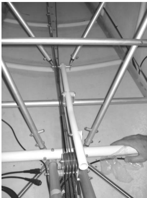
Figure 119 cable routing past flap handle.
