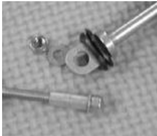
Figure 389 Upper fixing hardware. Note position of rubber grommet
