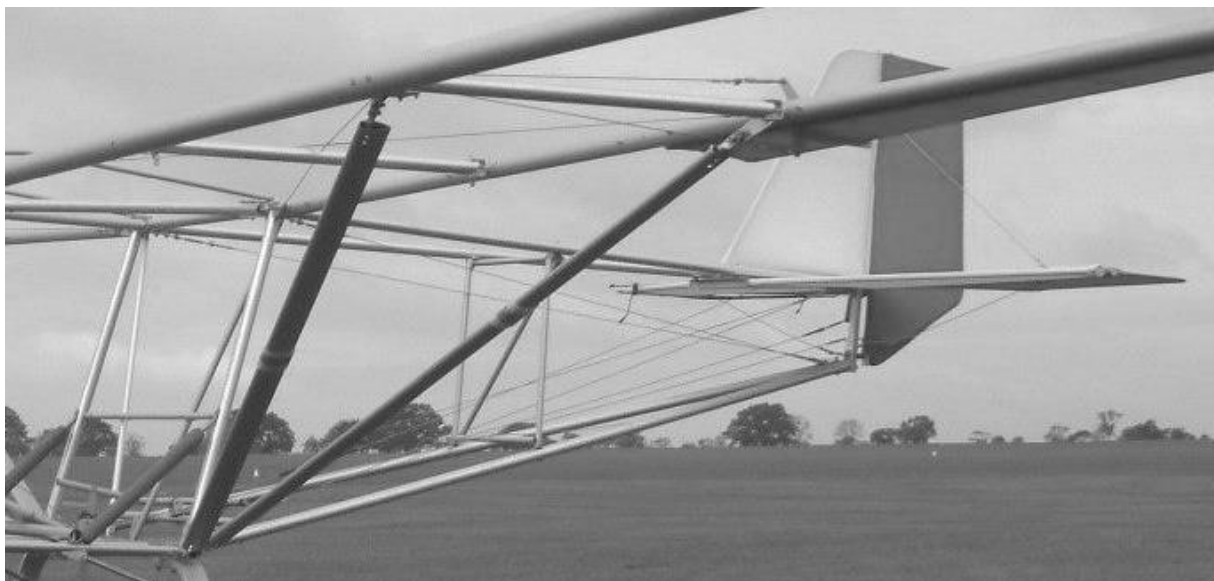
Figure 54 rear fuselage on uncovered frame.
