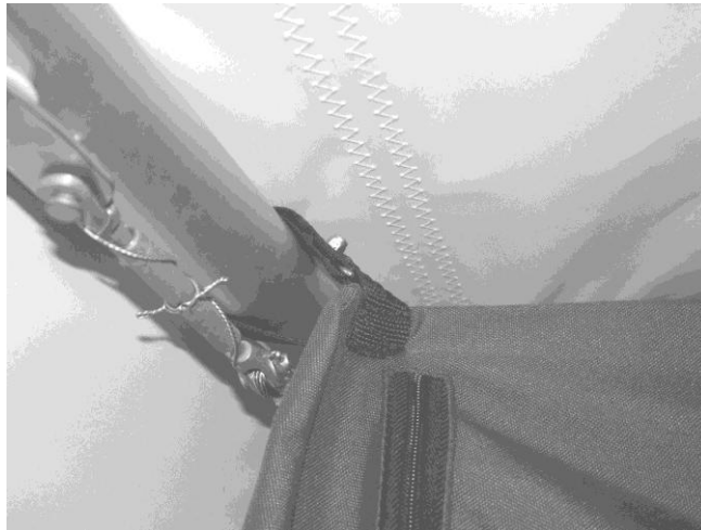
Figure 391 upper securing strap with Velcro and bolt.
