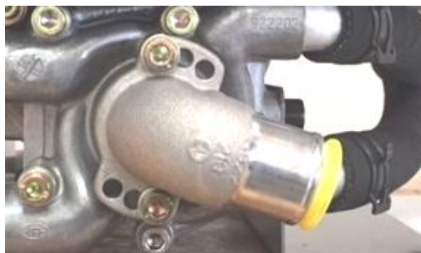
Figure 145 water pump outlet positioning
