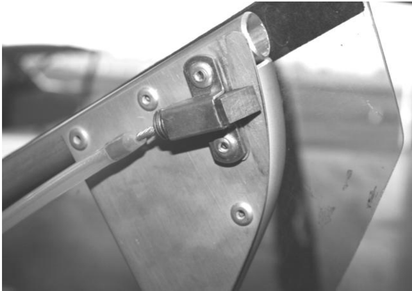
Figure 320 rear gusset plate and rear end of lower door.
