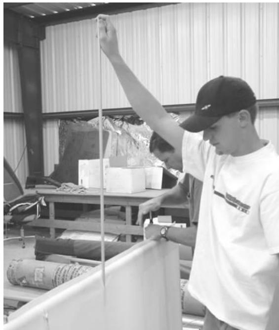
Figure 189 inserting a batten. Use your other hand to prevent the batten twisting.
