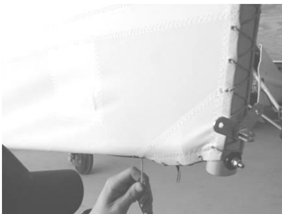
Figure 134 tighten the lacing.
