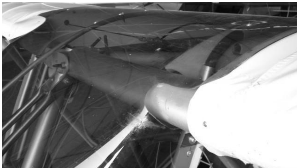
Figure 198 match up with wing so clear roof section will later fit flush like this
