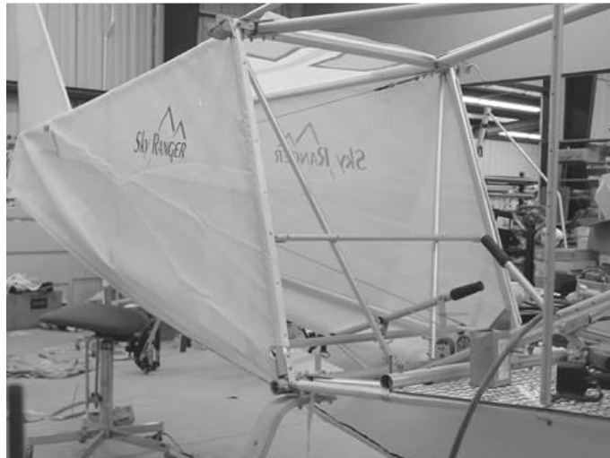
Figure 126 covering the fuselage.
