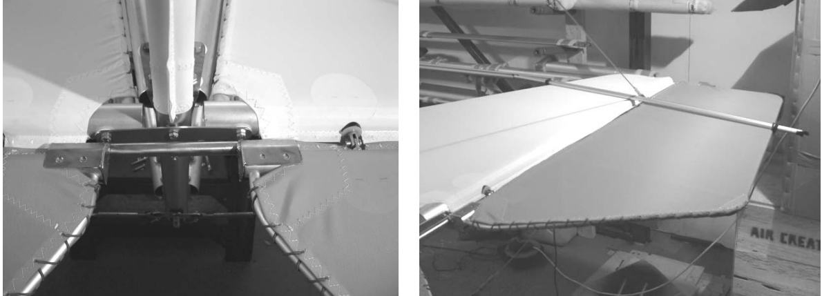
Figure 108 elevator joiner and alignment (note: Skyranger joiner shown – Nynja version has integral elevator horn).
