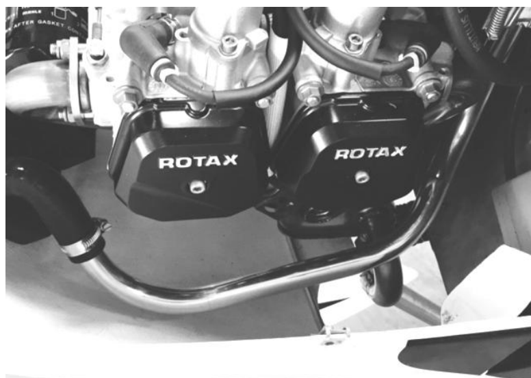
Figure 243 port water hose.
