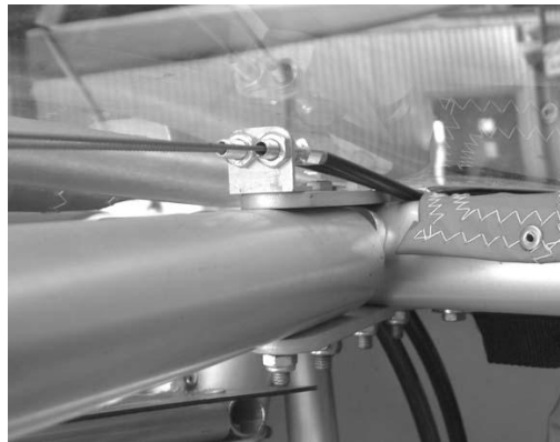
Figure 101 forward end of trimmer cables.
