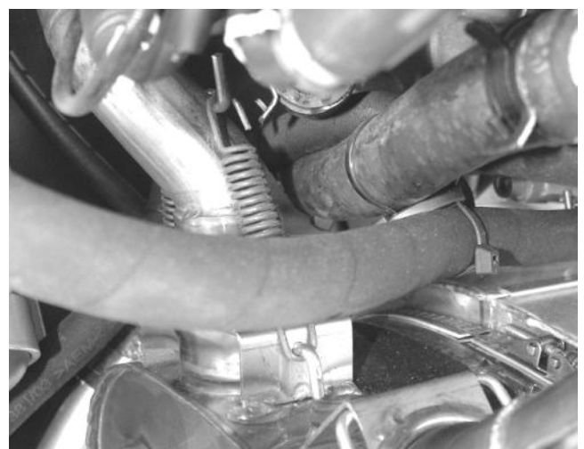
Figure 237 Routing of oil hose from Sump connection to inlet of oil tank. It should be cabletied up to the small water pipes under the engine in the position marked to keep it clear of exhaust.
