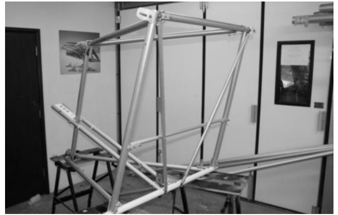
Twin TU19 tubes in position
