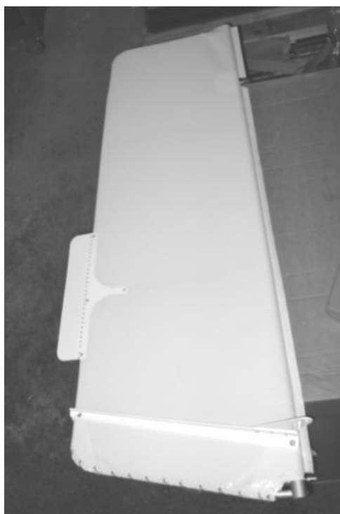
Figure 113 Swift 2 rudder (note: trim tab not required)
