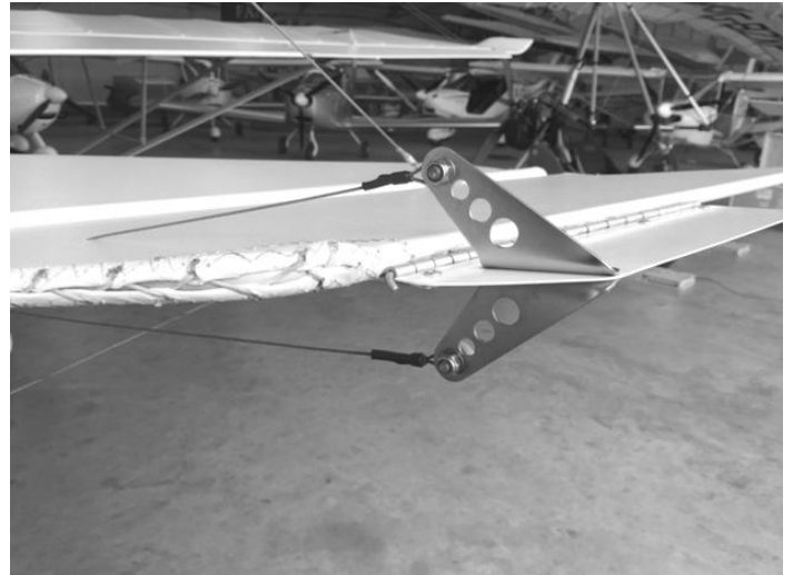
Figure 104 trim tab horns, aligned with cable bracket and hinge pin.
