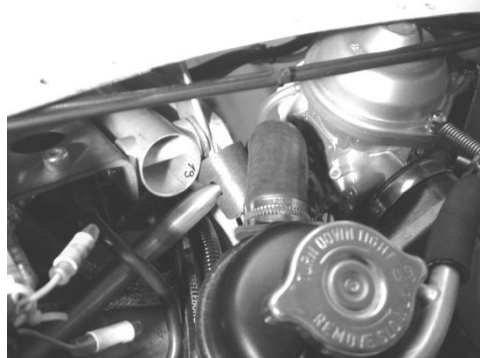
Figure 242 expansion tank and rubber elbow.
