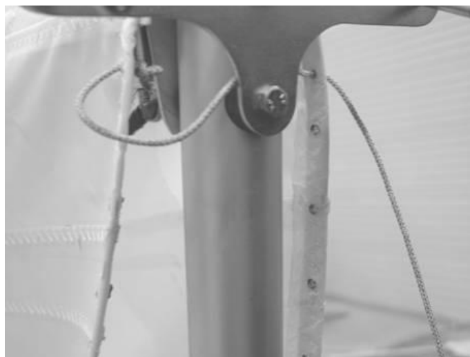
Figure 127 begin by loosely lacing the rear of the covering.
