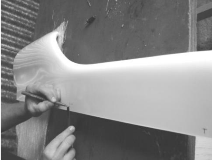
Figure 377 marking, drilling and fixing the winglet type wingtip fairings.
