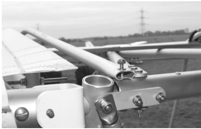
Figure 193 Rear ends of windscreen support frame
