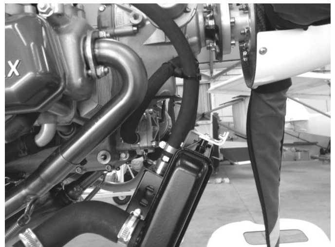
Figure 236 Hose routings from oil cooler outlets
