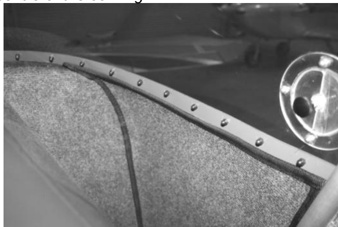
Figure 303 windscreen over lap inside cowling (note we painted the overlap to match interior fabric trimming.
