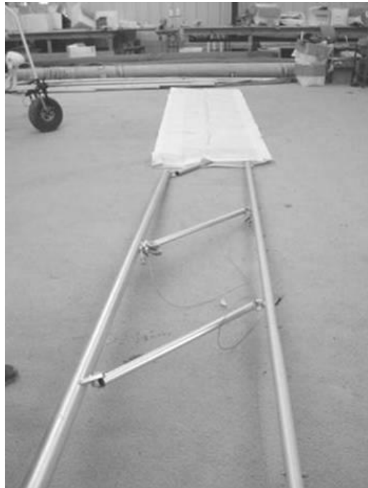
Figure 183 slide the wing frame into the covering.
