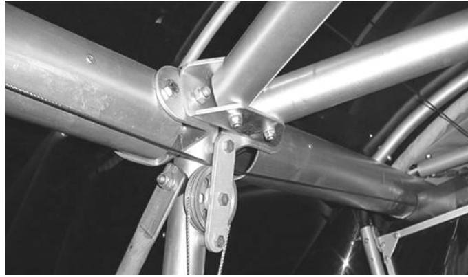
Figure 23 forward end of upper cabin triangle.
