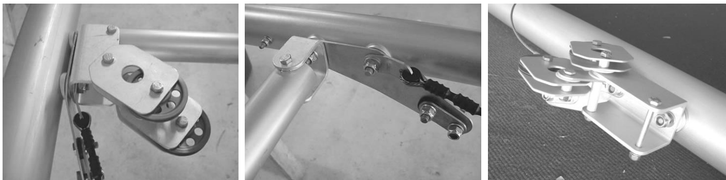
Figure 163 lift strut attachments and UKMOD aileron pulleys..
