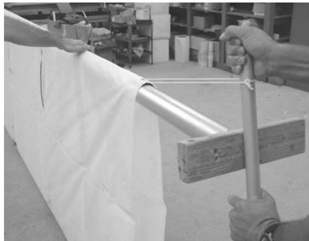
Figure 184 pulling the fabric into place.
