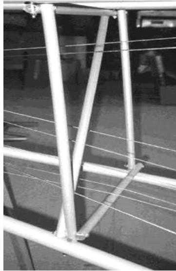
Figure 58 rear fuselage bracing frame, rear to left of photograph.
