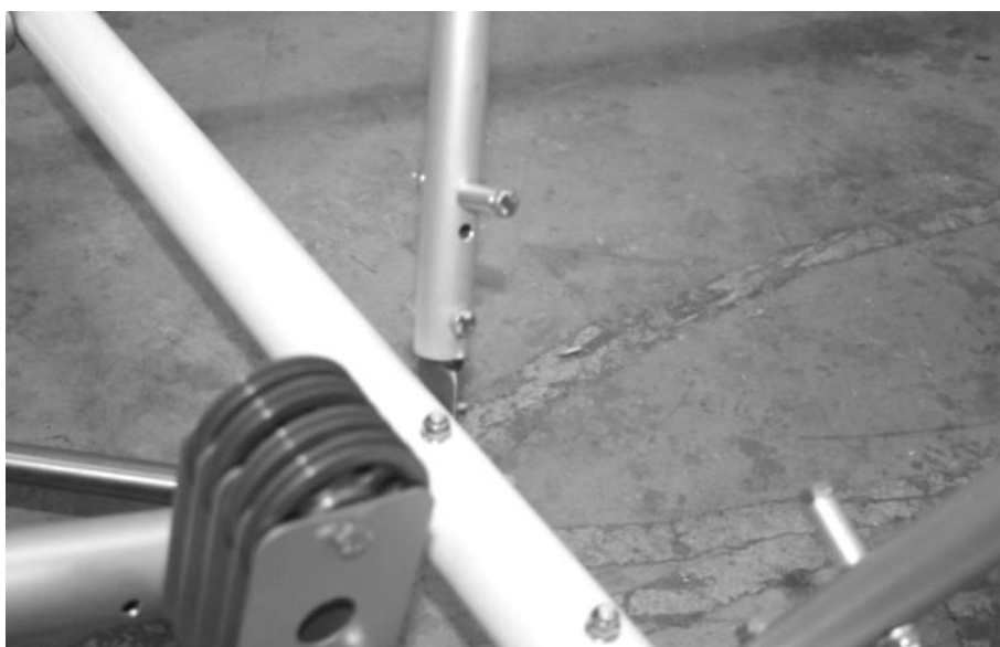
Figure 27 seat support peg.
