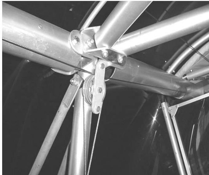
Figure 175 aileron cable fuselage pulleys.
