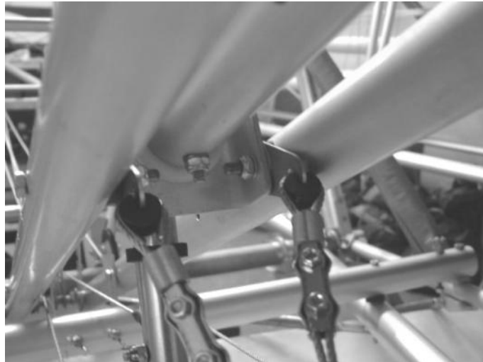
Figure 124 rudder stop cable adjustment.
