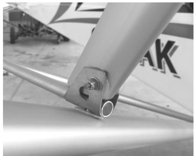
Figure 387 Rear and front lower fittings. Note orientation (looking from front)
