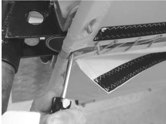
Figure 133 pulling the covering tight under the cabin.
