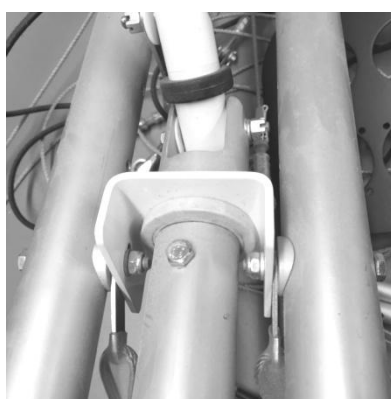
Figure 123 rudder stop cables attached to rear stick pivot.
