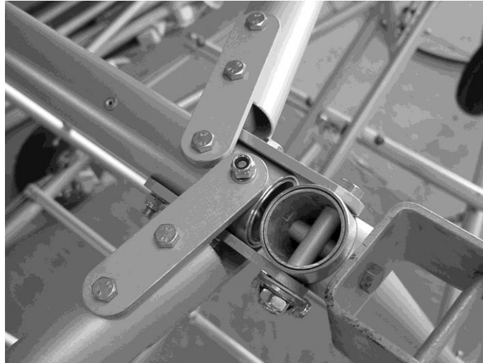
Figure 63 forward ends of upper tubes, rear to bottom left of photograph. d) Attach the lower tubes to the main undercarriage cross-beam, figure 6.
