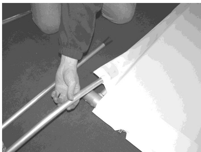
Figure 186 large diameter wing root battens.
