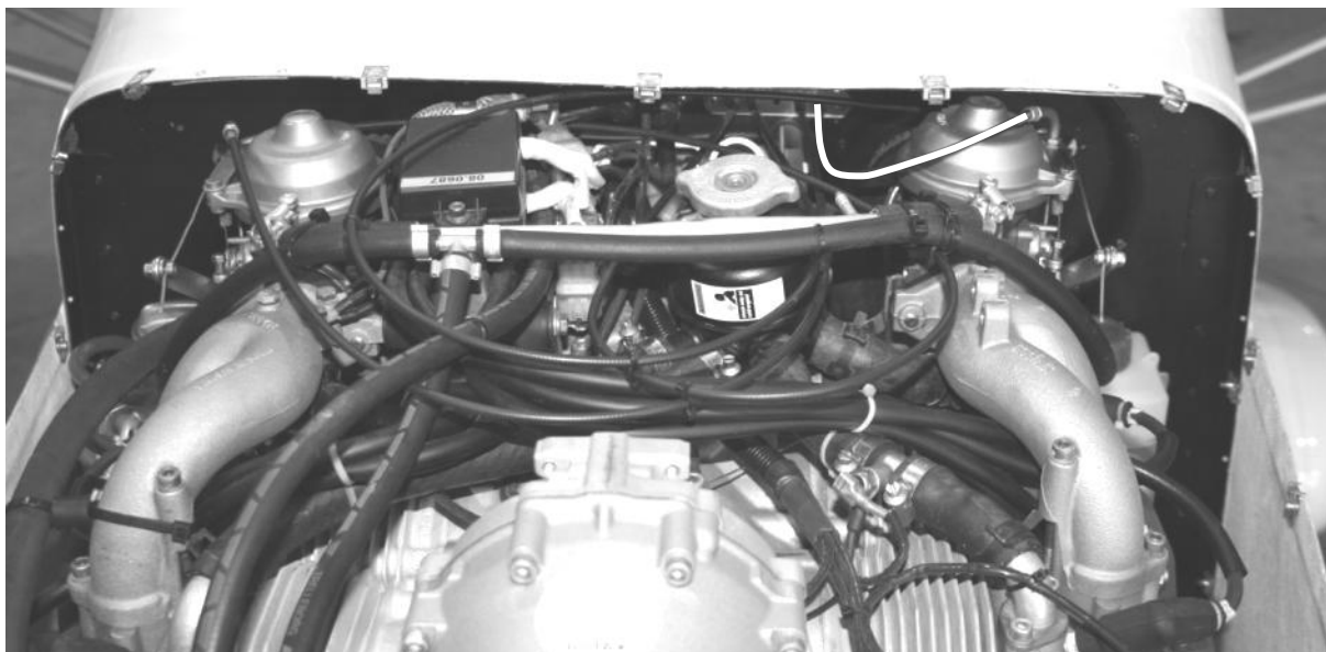
Figure 278 route of choke cable to port carburettor (in white)
