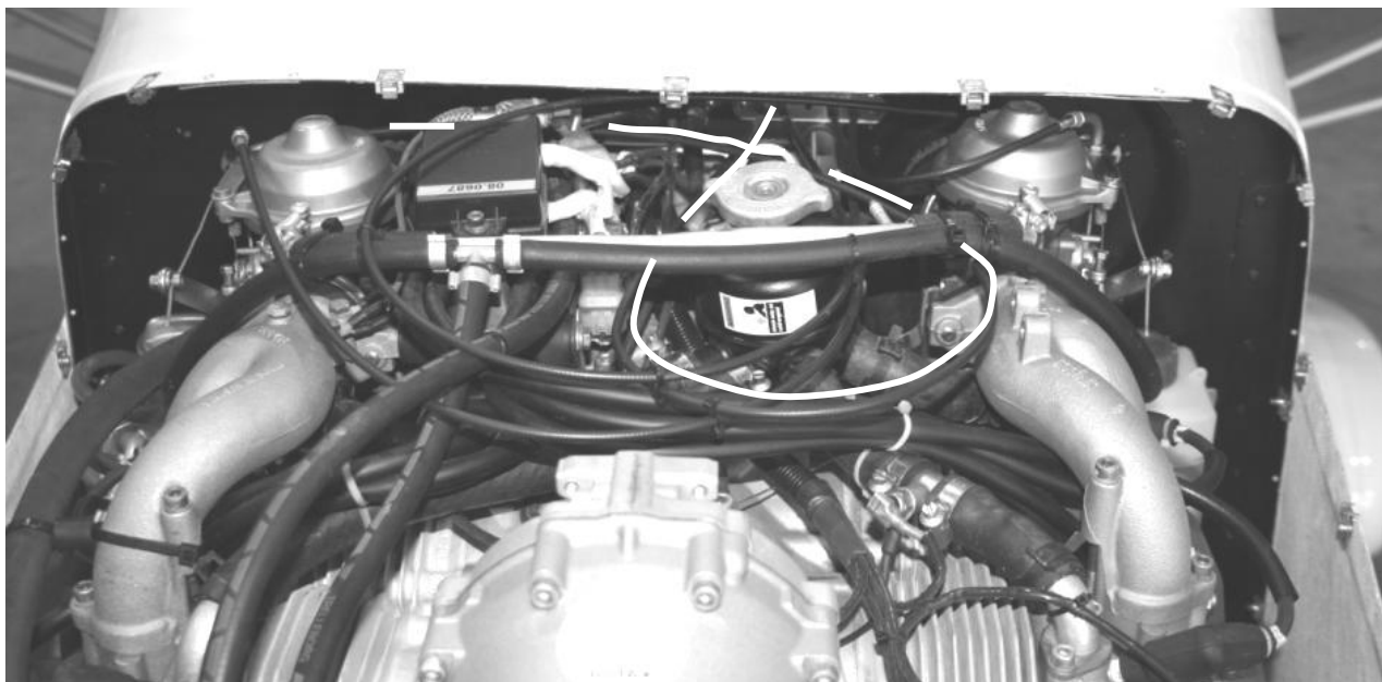
Figure 274 Route of throttle cable to starboard carburettor (in white)
