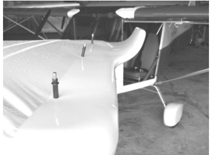
Figure 377 marking, drilling and fixing the winglet type wingtip fairings.
