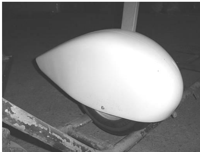
Figure 357 spat, showing outer mount bolt.
