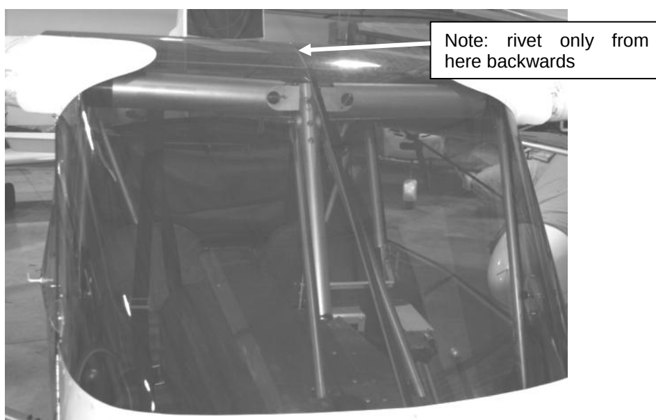
Fig 304 screen centre batten
