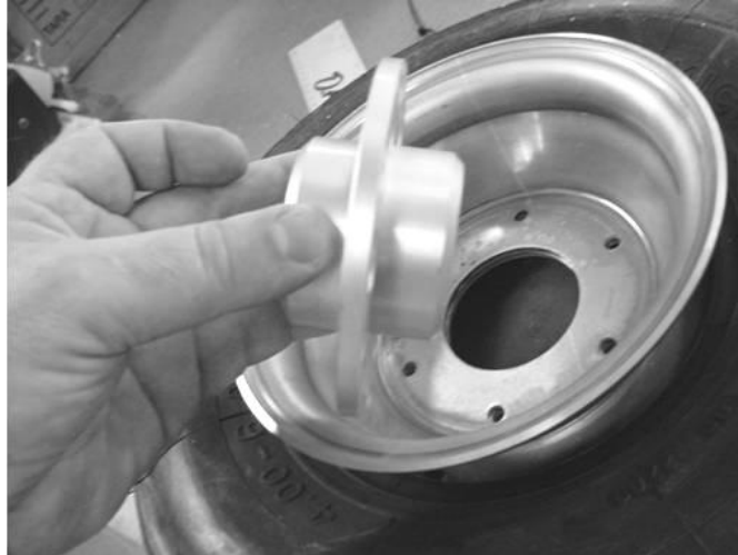
Figure 73 placing a hub against the wheel halves.
