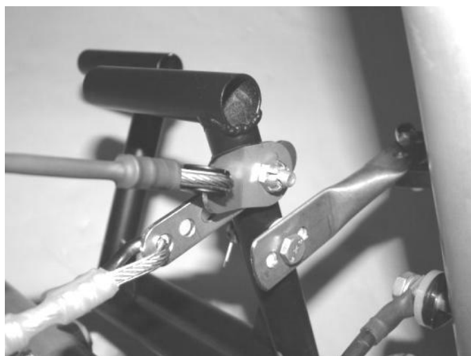
Figure 122 rudder stop cable tang fitted over rudder cable tang.
