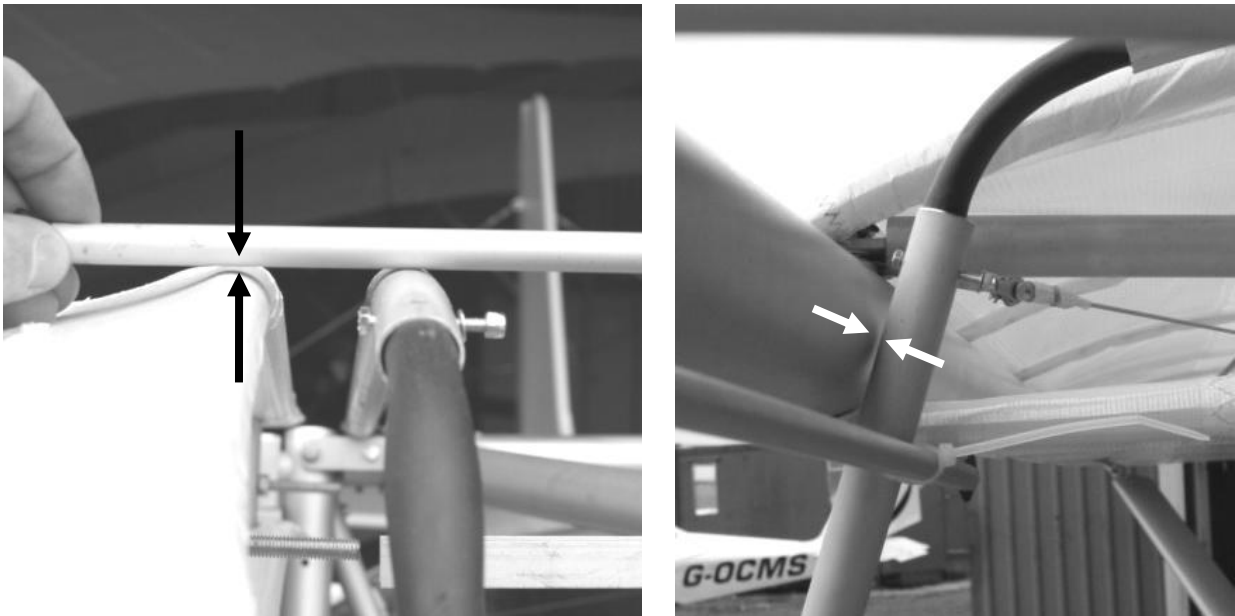
Figure 195 left – Check cabin roof tubes align with wing – level or slightly above. Right – check there is a gap of around 3-5mm here.
