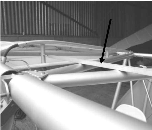
Figure 197 straight edge across cabin upper tubes. Measurement of 85mm from under tube to straight edge at point of max camber
