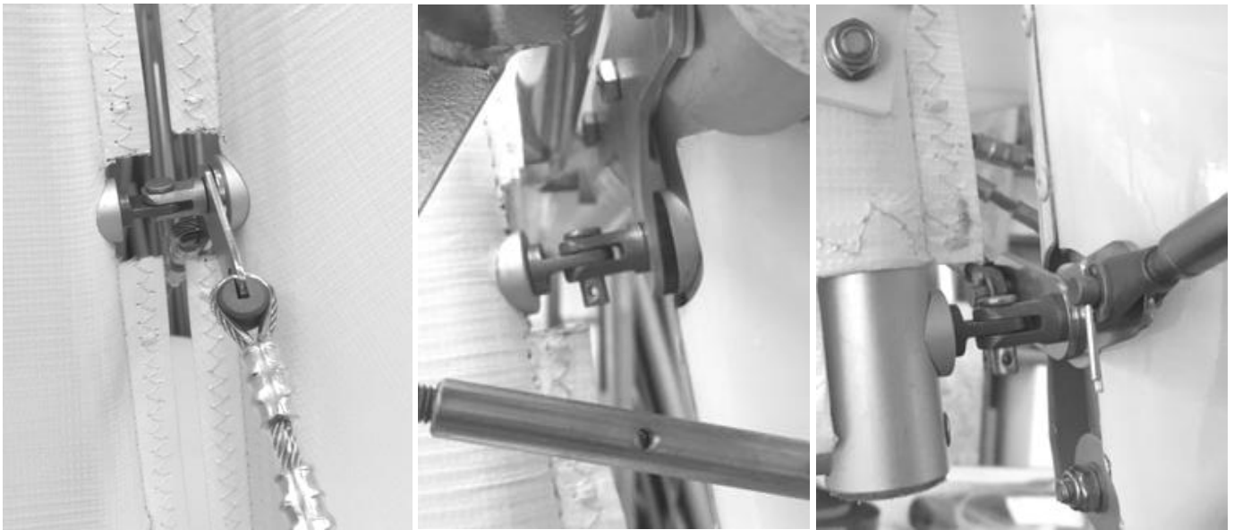
Figure 114 rudder mounting – top middle and lower hinge
